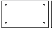
kit 102 V w 500 x h 300 x d 8mm w 19,69 x h 11,8 x d 0,31"
